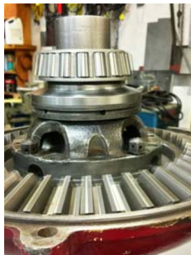
Spacer to replace original ball thrusts seen just below Timken bearing
