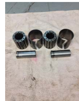
Wheel bearings which were replaced by the Lock Collar Ball bearings
