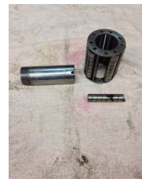
Pinion bearing and sleeve which were replaced by Torrington ones with a new sleeve
