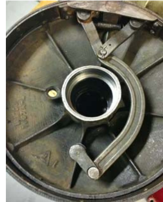
Stepped sleeve for new style wheel bearing
