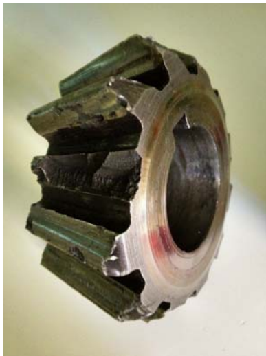
Broken Pinion Not very pretty!
