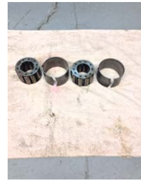
Carrier Hyatt bearings which were replaced by Timken ones
