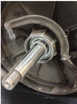
New style Lock Collar Ball wheel bearing
