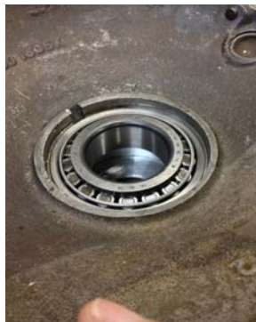
Timken bearing in rear end housing
