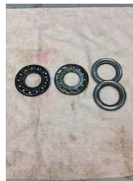
Carrier thrust bearings, also replaced by the Timken bearings
