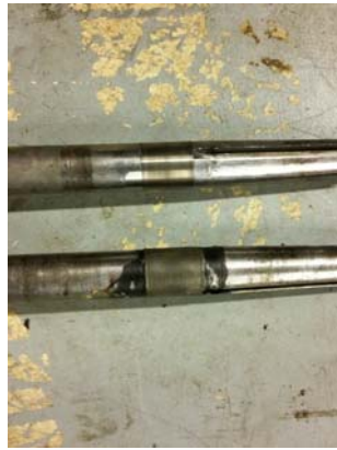
Axle spray welding to fit new style bearings. Bottom axle before grinding and the top one is after
