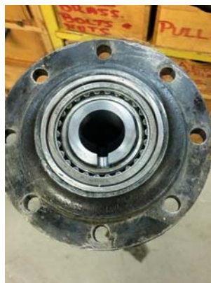
Torrington pinion bearings with new sleeve installed
