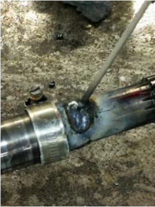
Drive shaft straightening
