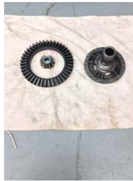
Crown, pinion and crown gear half of the carrier
