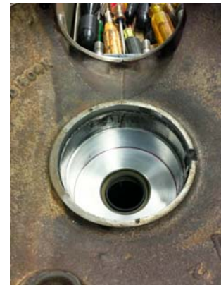
Stop for Timken cup and new seal and plate
